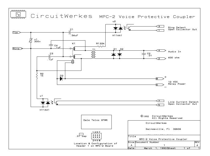
Figure 1. The MPC-2's Schematic diagram.
