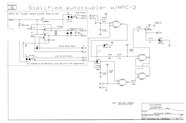
Sample schematic for making an automatic coupler using an MPC-2.
