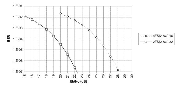
Figure II-1 Bit Error Rate as a Function of Eb/No for 2 and 4 Level FSK
