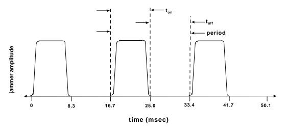
Figure I-3 Microwave Oven Magnetron Duty Cycle
