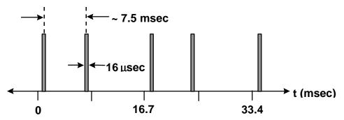
Figure II-3 Time Domain Representation of MWO Interference for Condition B
