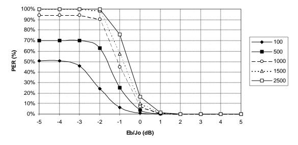
Figure III-4 DSSS PER as a Function of Packet Length (bytes) and Relative Jammer Power @ 1 Mbps
