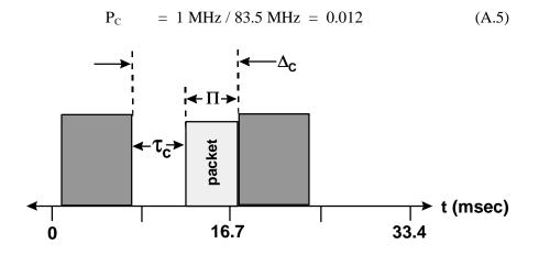
Figure A-3 MWO Interference Pulses (Condition C)
