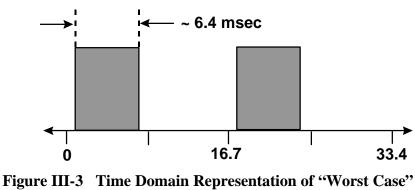
**MWO Interference in a DSSS System**
