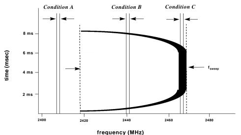
Figure A-1 Possible Conditions for Occupied Channel in Presence of MWO Interference
